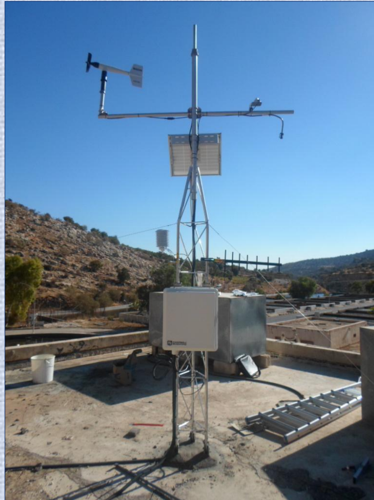
Automatic Weather Station, University Of Jordan, Amman.
